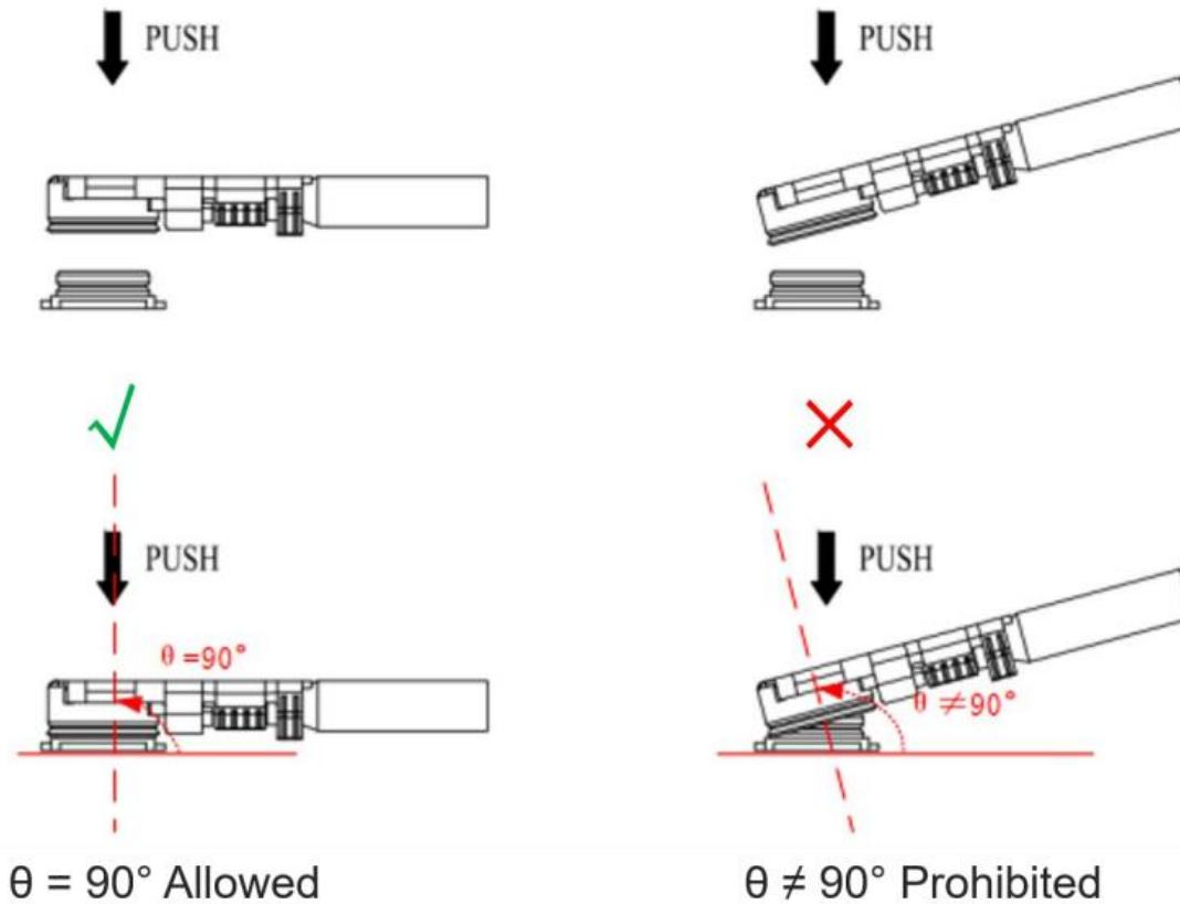
The illustration of pulling out the coaxial cable plug is shown below,  $\theta = 90^\circ$  is acceptable, while  $\theta \neq 90^\circ$  is not.
