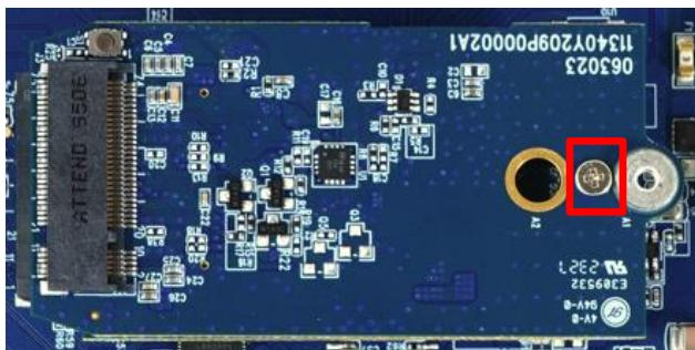
Step 3: Fasten the module to the main board of MDG230 by a screw boss.
